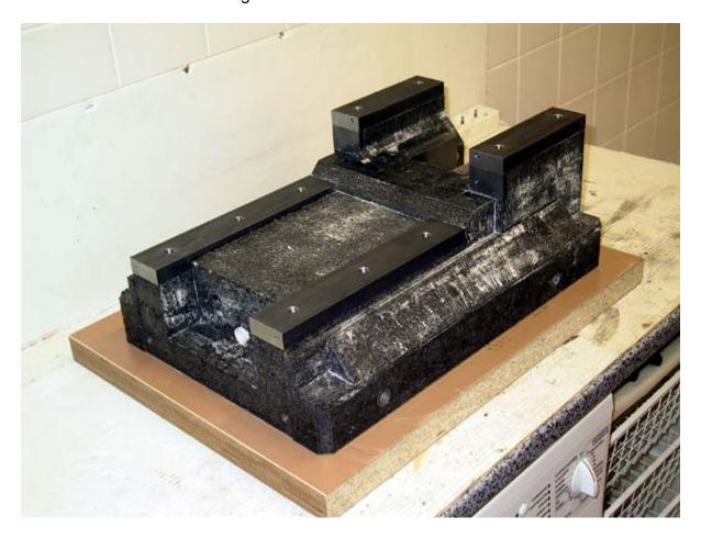
Front of the base. Note the precision steel pieces cast in place...
