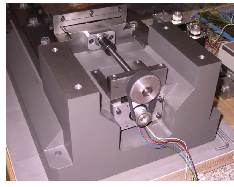
Painted and assembly underway. The Y-Axis mechanism is under the column. That much solid epoxy granite has got to make for a more rigid machine than the normal hollow cast iron!
