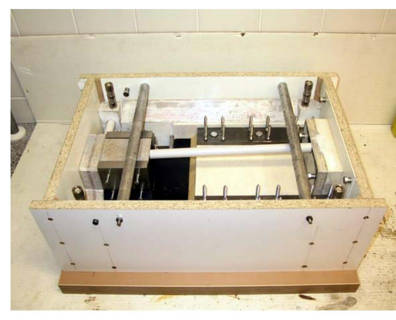
Mold for the base. This base will be case upside down. Note the screws sticking up from the metal parts--that's how they're anchored into the epoxy matrix...
