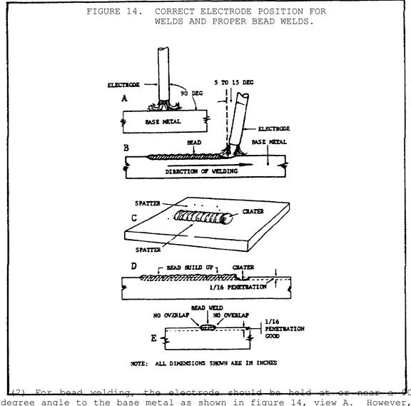
degree angle to the base metal as shown in figure 14, view A. However, in order to obtain a clearer view of the molten puddle, crater, and arc, the electrode should be tilted between 5 and 15 degrees toward the direction of travel as shown in figure 14, view B.
