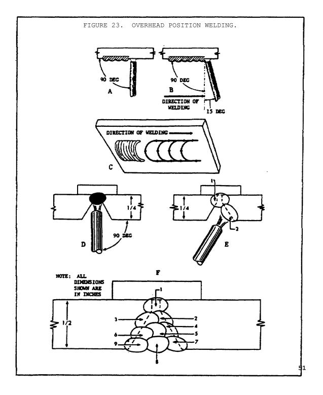
down or sag on the plate. If the arc is too long, the difficulty in transferring metal from the electrode to the base metal is increased and large globules of molten metal will drop from the electrode and the base metal. This action can be prevented by first shortening and then lengthening the arc at intervals. Care must be taken not to carry too large a pool of molten metal in the weld.
