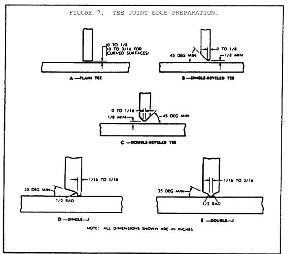
c. Types of Welds. The type of weld used will determine the manner of seam, joint, or surface preparation. A listing of the different welds used is provided in the following subparagraphs.
