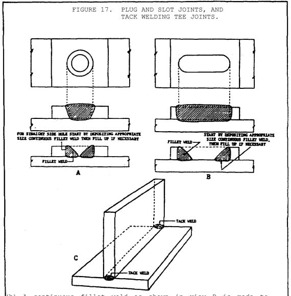
(b) A continuous fillet weld as shown in view B is made to obtain a good fusion between the sidewalls of the hole or slot and the surface of the lower plate. The procedure for this fillet weld is the same as for lap joints, which will be described in paragraph 5g(2) on page 45. The hole or slot is then filled in to provide additional strength in the weld.
