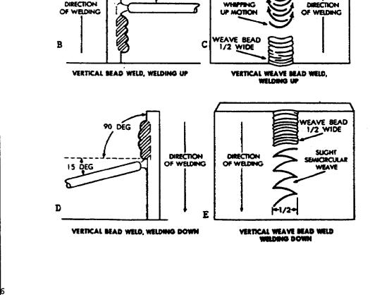
(d) When welding upward, the electrode should be held at 90 degrees to the vertical as shown in figure 20, view B, on the previous page. When welding upward and weaving is necessary, the electrode should be oscillated as shown in figure 20, view C.
