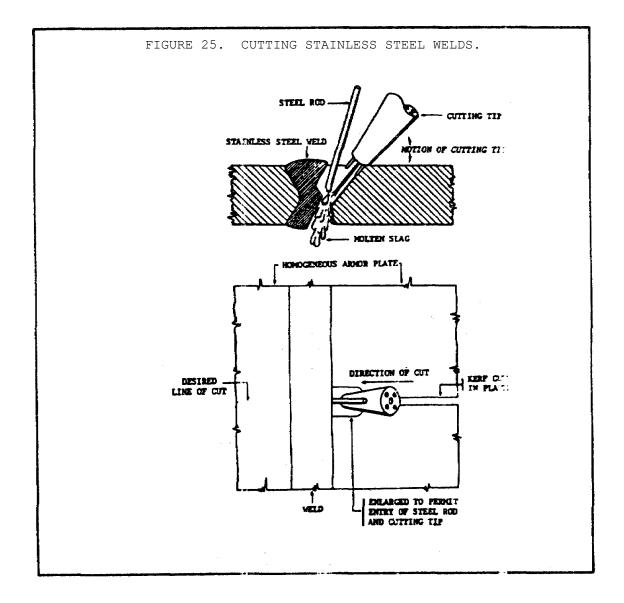
(c) Cracks or other defects on the face of stainless steel welds can be removed by holding the cutting tip at a slight angle away from the face of the weld as shown in figure 26. The reaction between the cutting oxygen and the steel rod develops sufficient heat to melt the weld metal and is then washed away. Afterwards, the joint surface can be rewelded.
