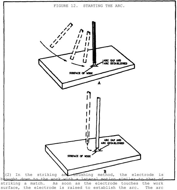
surface, the electrode is raised to establish the arc. The arc length or gap between the end of the electrode and the work should be approximately equal to the diameter of the electrode. When the proper length of the arc is obtained, a sharp crackling sound can be heard.
