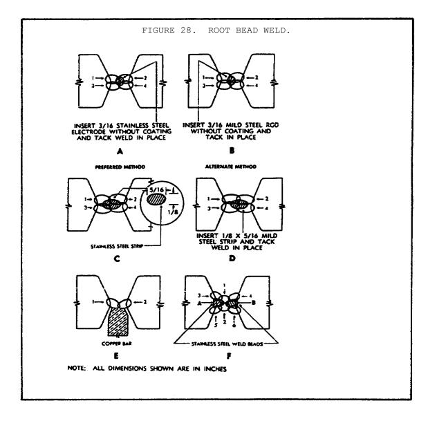
method, shown in figure 28, view D, on the previous page, uses a mild steel strip. When this method is used, the backing rod or strip should be chipped out before depositing beads 3 and 4.
