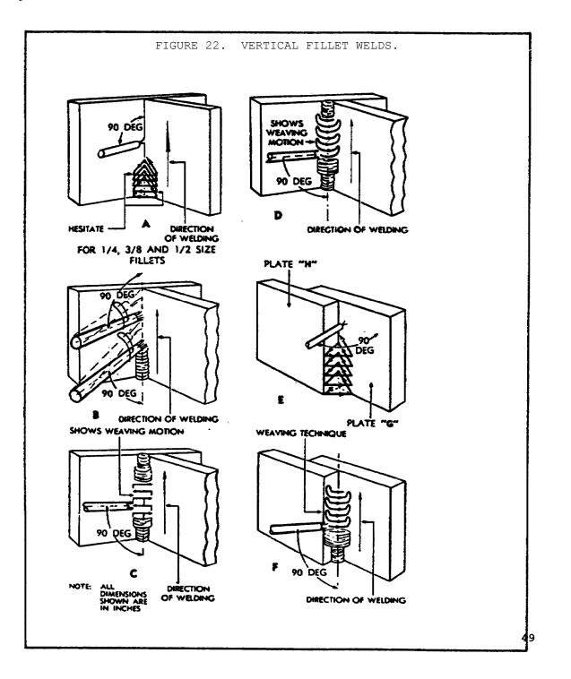
more than 15 degrees above the horizontal for proper molten metal control. The arc should be held short to obtain good fusion and penetration.
