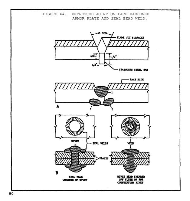
by 1/4 inch stainless steel bar which is placed in the damaged portion of the armor plate. It is then bead welded in place. The principal advantages of this joint are its simplicity, and good structural and ballistic properties. Care should be taken that no welding is done on the hard face side of the armor plate.
