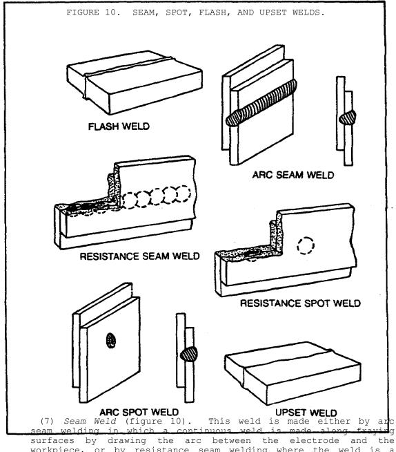
workpiece, or by resistance seam welding where the weld is a series of overlapping spot welds made progressively along a joint by rotating the circular electrodes.
