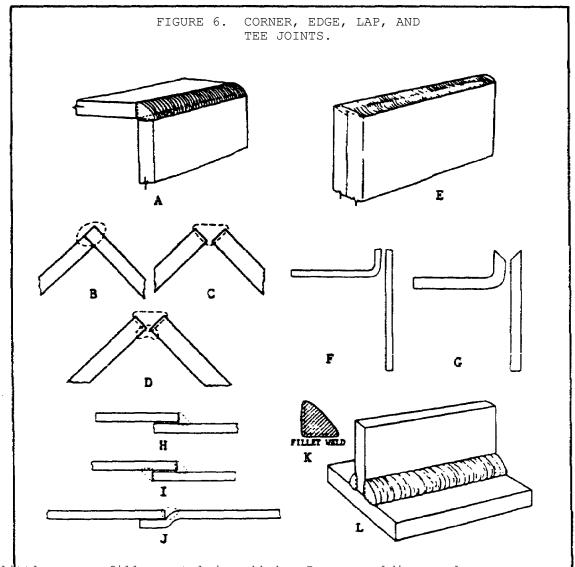
little or no filler metal is added. In arc welding, only a very light bead is required to make the joint. The open corner joint, shown in figure 6, view C, is used on heavier sheets and plates; the two edges are melted down and filler metal is added to fill up the corner. Corner joints on heavy plates are welded from both sides as shown in figure 6, view D. The joint is first welded from the outside, then reinforced from the back side with a seal bead.
