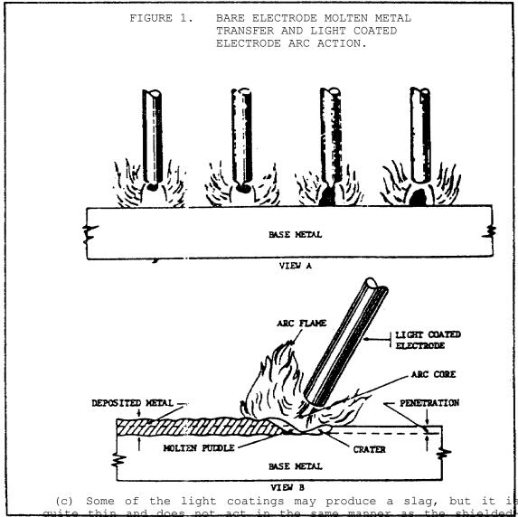
arc, slag-type electrode. The action of an arc obtained with a light-coated electrode is shown in figure 1, view B.
