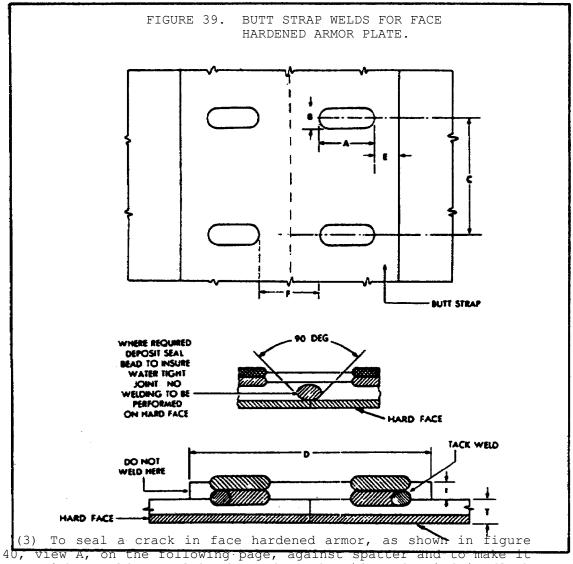
watertight, weld a seal bead on the soft side and grind it flush before applying the butt strap. All welding should be performed on clean, scale free surfaces. Previously deposited weld metal should be thoroughly cleaned by chipping and wire brushing to remove slag and oxides to ensure sound welds.
