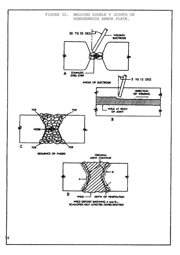
Excessive dilution will cause the weld to be non-stainless, brittle, and subject to cracking. Proper penetration will give a long scalloped heat affected zone on each side of the weld as shown in figure 32, view D, on the previous page. Insufficient penetration (surface fusion) will produce a fairly straight edged heat affected zone on each side of the weld. This condition is undesirable from the standpoint of good ballistic properties.
