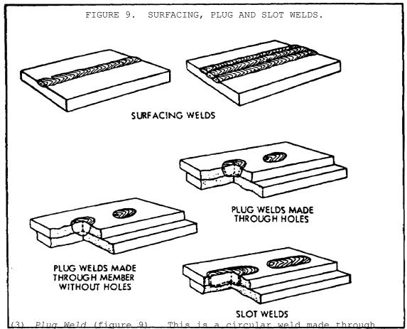
one member of a lap or tee joint joining that one member with the other. This type weld may or may not be made through a hole in the first member.
